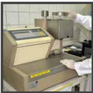
Fig : 7.5 Melt Mass Flow Rate Test
