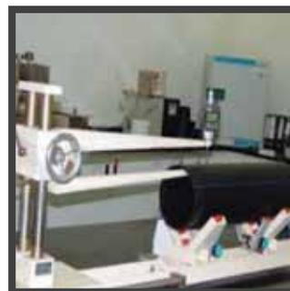
Fig : 7.9 Wall Thickness and Outside Diameter Measurement
