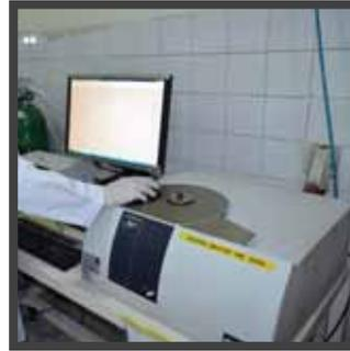
Fig : 7.7 Thermal Stability Oxidation Induction Time Test(OIT)
