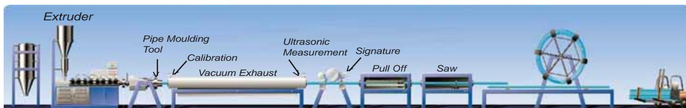
Fig 5.1.a : Extruder Machine for HDPE Pipes
