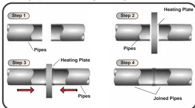
Fig : 11.1.c Butt Welding Process
